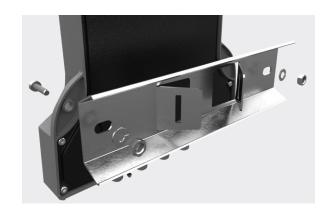
Once bracket is secured to the OTx open jubilee clip thread through slots as shown right, attach around mast and tighten using a flat bladed screwdriver.
