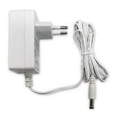
**12V 1.5A power supply** with **male jack connector** (2.1 x 5.5 x 12mm; inner positive, outer negative) and European plug.
