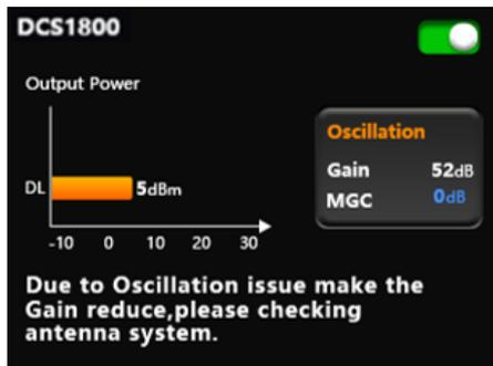
Repeater system will strictly check Self-oscillation degree for all of sub-band and firstly will show abnormal status (Orange) in Menu page, ISO and ALC function would auto generate and if user enter into the soft Self-oscillation sub-band, user could check more details about Self-oscillation with recommend info.
