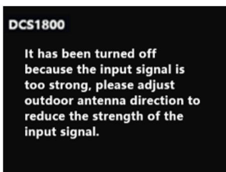
This system auto-generate message caused by excessively strong signals from cell tower, referring to below troubleshooting sections.
