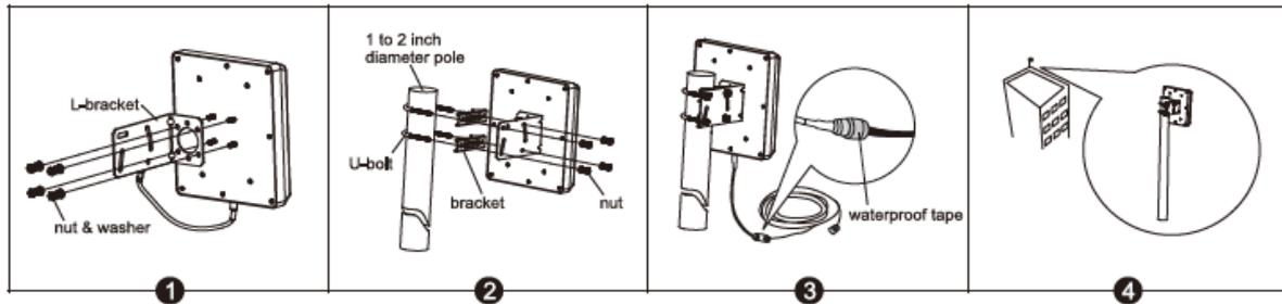
**Note:** Wrap waterproof tape around the connectors between outdoor antenna and feeder line to avoid water or other kinds of damage.
