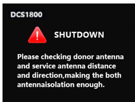
if not working and Self-oscillation get seriously, which overcome ISO and ALC function address range ( $ALC \geq 42\text{dB}$ ,  $ISO \geq 42\text{dB}$ ), the Sub-band (with Self-oscillation) would be auto-shutdown as above message, which shows shutdown status (red) for this Sub-band in Menu Page, to protect Base Station wouldn't get interference.
